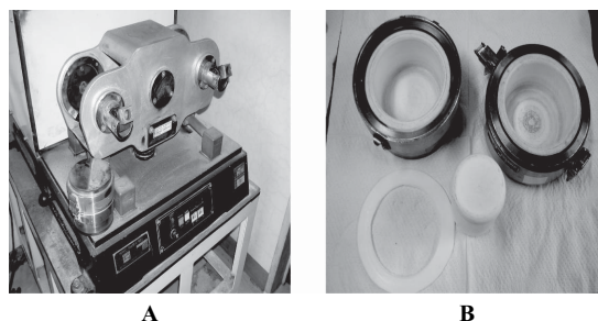
FIGURE 2. Photographs of the apparatus (A) and grinding cell (B) of vibrating rod mill (TI-200, Heiko Seisakusho, Tokyo, Japan).
